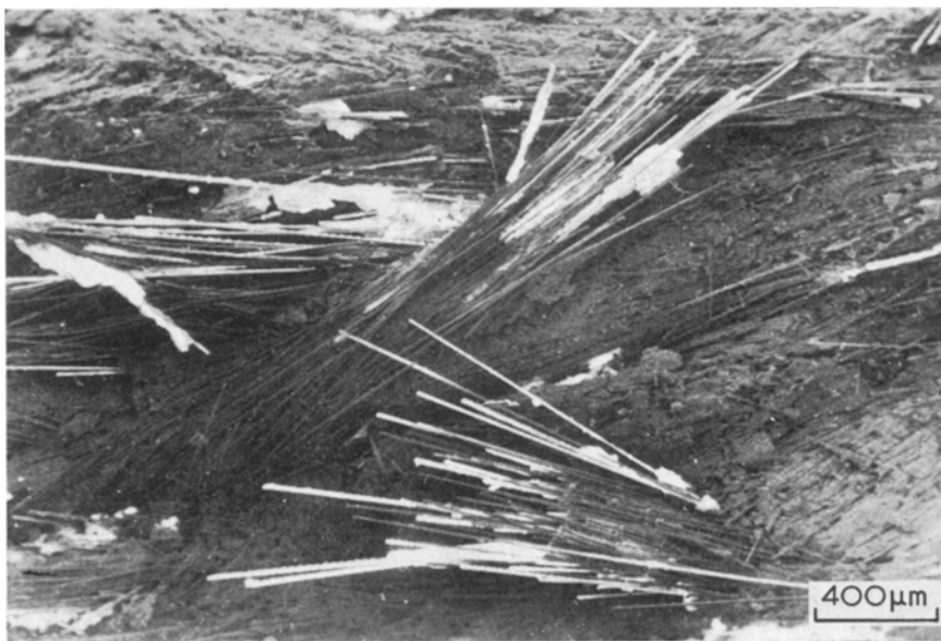
Figure 2 Scanning electron micrograph of a fracture surface in a specimen of a dough moulding compound which shows the non-uniform distribution of glass fibres.
